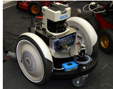
Fig. 5. Segway RMP-50 equipped with embedded computer, SICK laser range finder, GPS receiver, magnetometer, gimbaled pyrometer and wireless communication.
