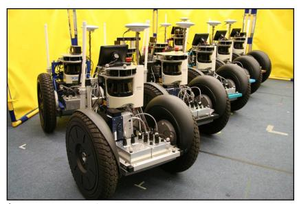
Segway RMP50/50XL outdoor robot fleet, equipped with Septentrio GPS, 180 deg FOV SICK and 270 deg FOV Hokuyo Lidar, Mimo touchscreen interfaces, Firefly Cameras, onboard IMU, mobile WiFi, custom electronics and mounting hardware.
