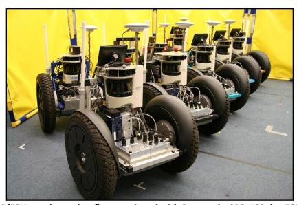
Segway RMP50/50XL outdoor robot fleet, equipped with Septentrio GPS, 180 deg FOV SICK and 270 deg FOV Hokuyo Lidar, Mimo touchscreen interfaces, 3x Firefly Cameras, onboard IMU, mobile WiFi, custom electronics and mounting hardware.
