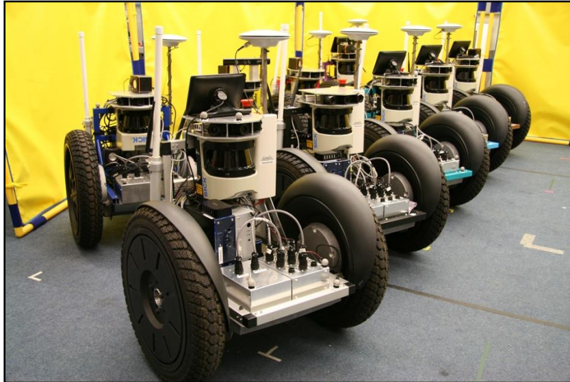
Segway RMP50/50XL outdoor robot fleet, equipped with Septentrio GPS, 180 deg FOV SICK and 270 deg FOV Hokuyo Lidar, Mimo touchscreen interfaces, 3x Firefly Cameras, onboard IMU, mobile WiFi, custom electronics and mounting hardware.
