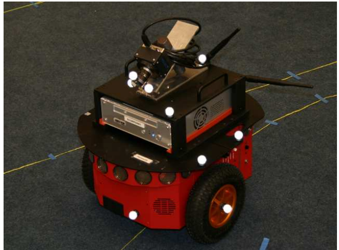
Figure 1. Pioneer 3-DX rover with custom camera mounting. The luminous circles are retro-reflectors used for motion capture. The sonar panels on either end of the rover were not used during this study.
