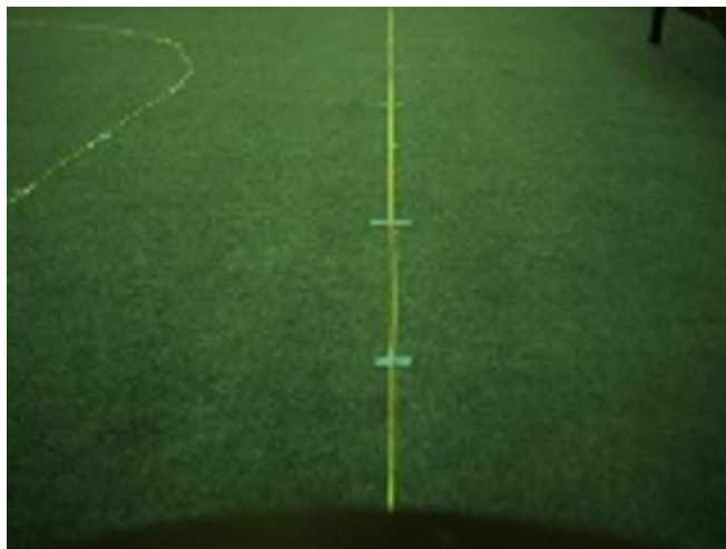
Figure 2. Example of a camera image seen by subject at the beginning of a lap. The yellow line is the reference route the subject has been instructed to follow. The models presented in this paper assume that subjects ignore later sections of the route that may come into view as seen in the upper left.
